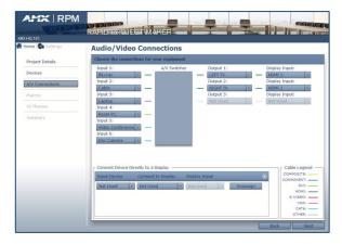
3. Select source devices and their destination to route audio and video to the desired input or output on the AV switcher. You can also bypass the switcher by assigning a device to connect directly to a display.
